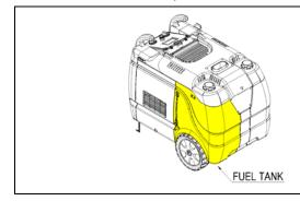
Open the black-colored fuel tank cap on the right side and fill the tank.
