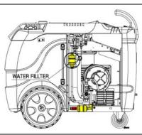
1. Close the Water filter shut off valve.
