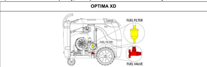
1. Close the Fuel filter shut off valve..
