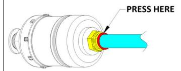
3. Rotate the water filter counterclockwise to detach it.
